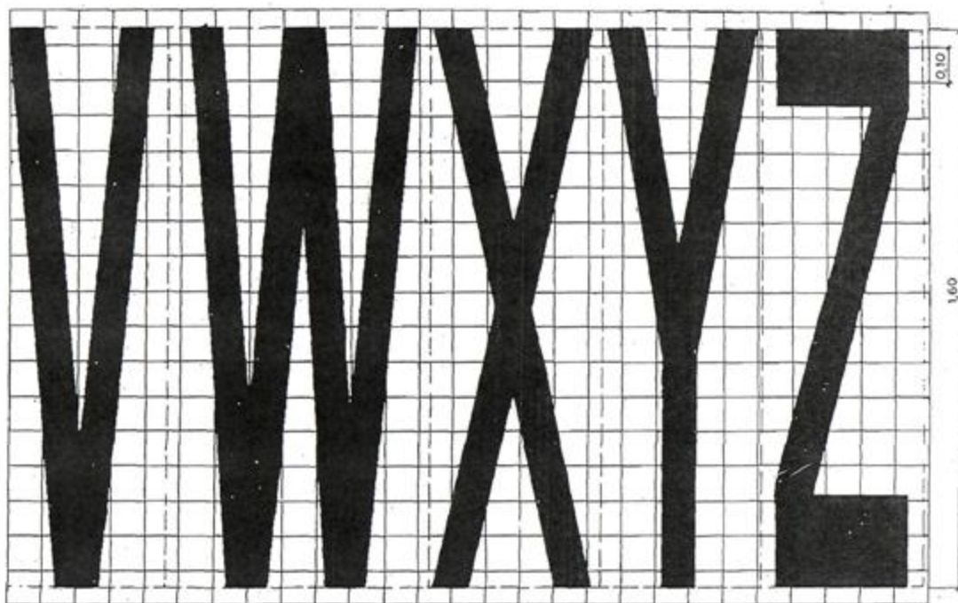
Letter markings for roads with a speed limit of 60 km/h or less. measures in meters
